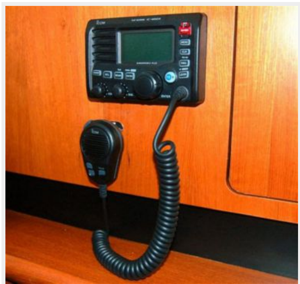
Salon VHF with Intercom to Bridge
