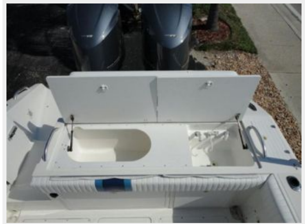
Livewell/Sink under Aft Seating
