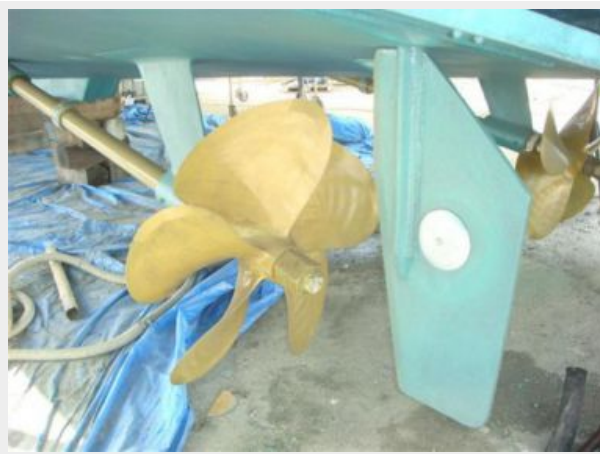
78' Buddy Davis port running gear
