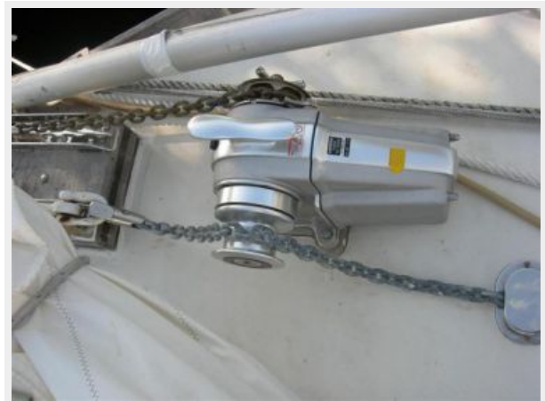
Electric anchor windlass with remote contro-
