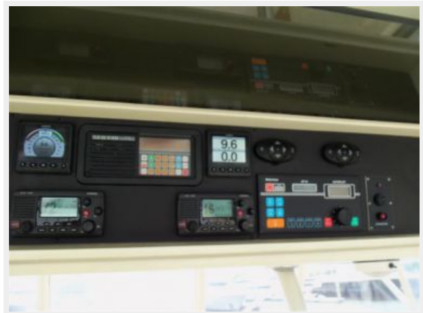
Overhead Box Detail
