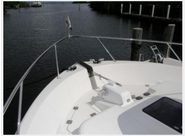
Windlass & Anchor Roller
