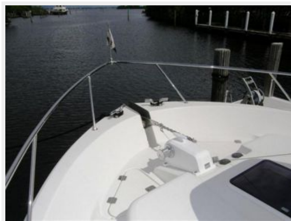
Windlass & Anchor Roller
