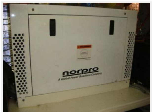
44' North Shore Trawler generator sound box
