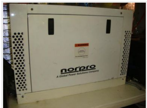
44' North Shore Trawler generator sound box
