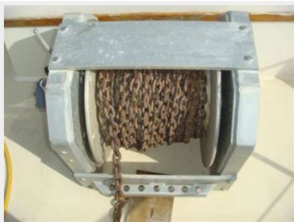
44' North Shore Trawler anchor windlass
