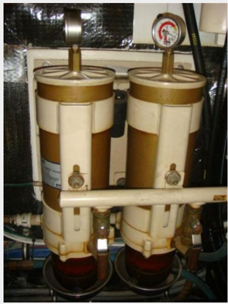
70' Hatteras Motoryacht Racor fuel filters
