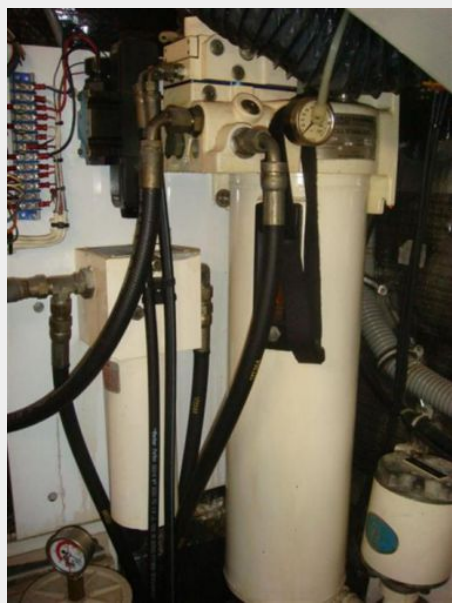
70' Hatteras Motoryacht Naiad stabilizer hydraulic pak
