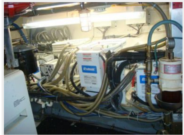
70' Hatteras Motoryacht air conditioning compressors
