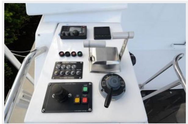
Pilothouse Aft Deck Controls
