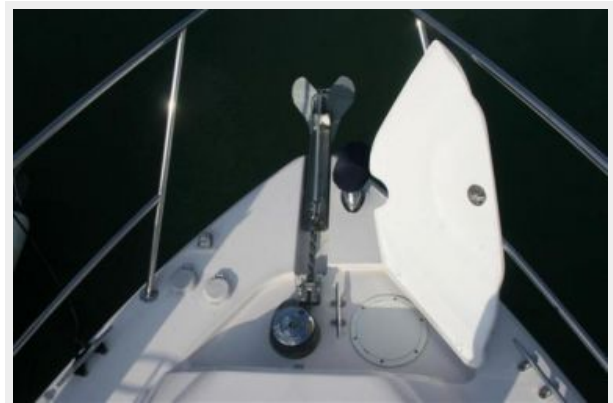
Foredeck anchor locker & windlass
