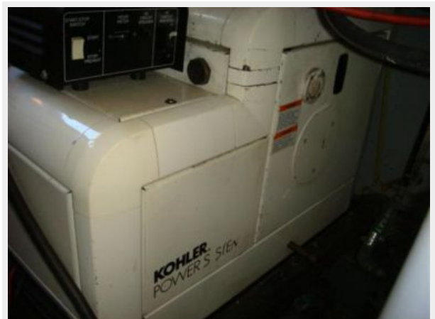
41' Symbol generator soundbox
