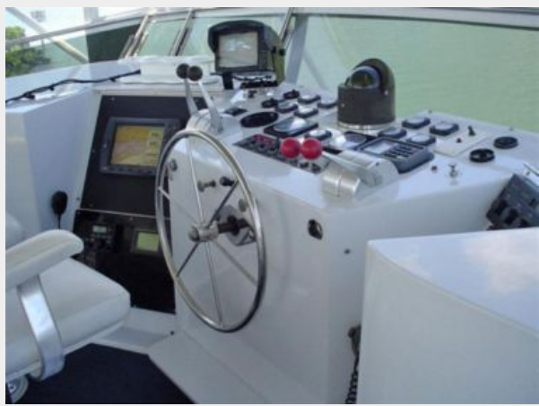
Bridge Deck Helm Station
