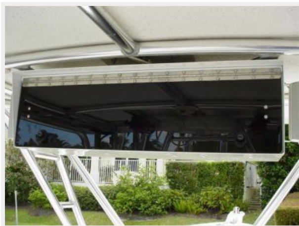
Overhead Electronics Box
