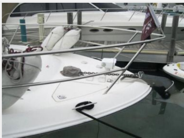
Bow, Windlass and Remote Spotlight
