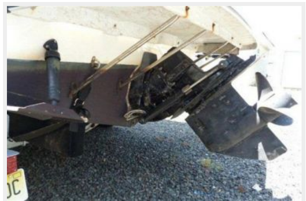
Engine and Mechanical Equipment 5 - Outdrive
