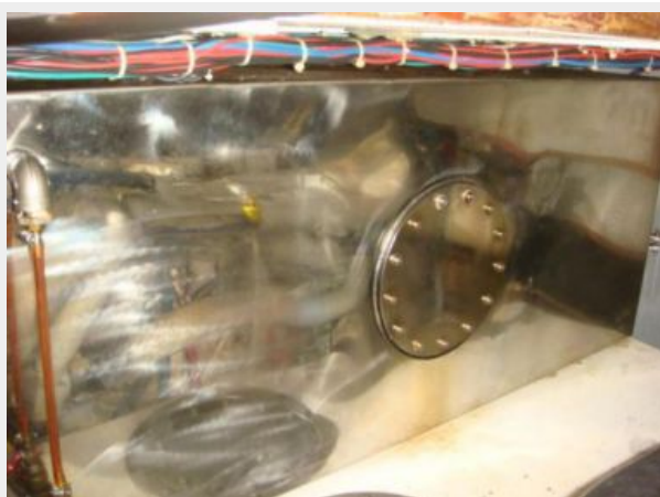
43' Sterling Atlantic starboard fuel tank
