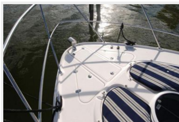
Bow Anchor Lockers and remote Spotlight
