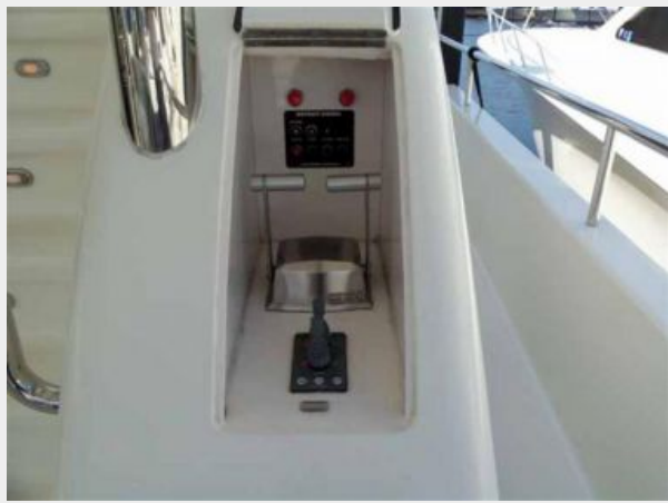
One of Two Aft Deck Docking Stations
