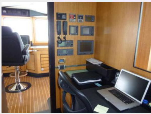
Wheelhouse radio room
