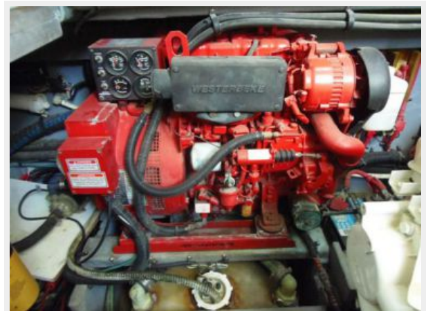
Sea Ray 370 aft cabin genset
