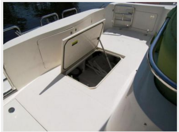
Electric Hatch to Cockpit Lazarette
