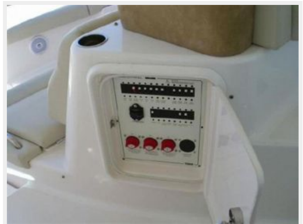
Cockpit Electric Control Panel
