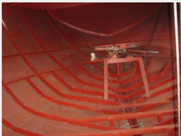
interior - aft - rudder quadrant ( master berth was built over this quadrant)
