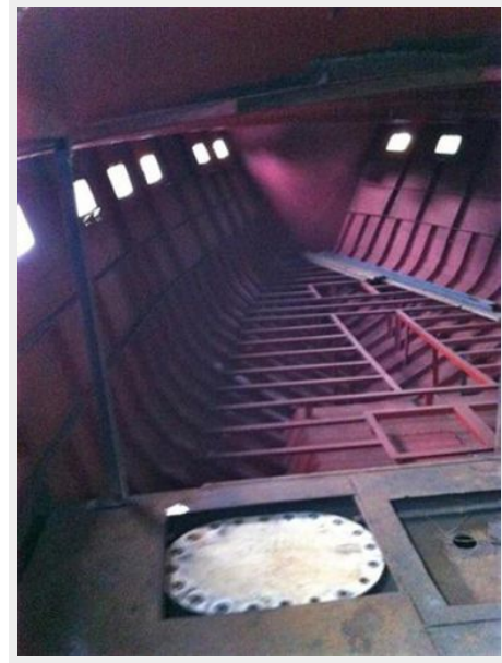
interior forward & top of fuel tank
