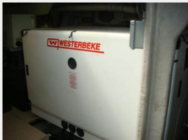
54' Sea Ray generator sound box
