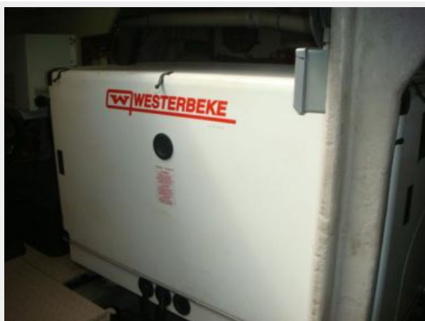
54' Sea Ray generator sound box
