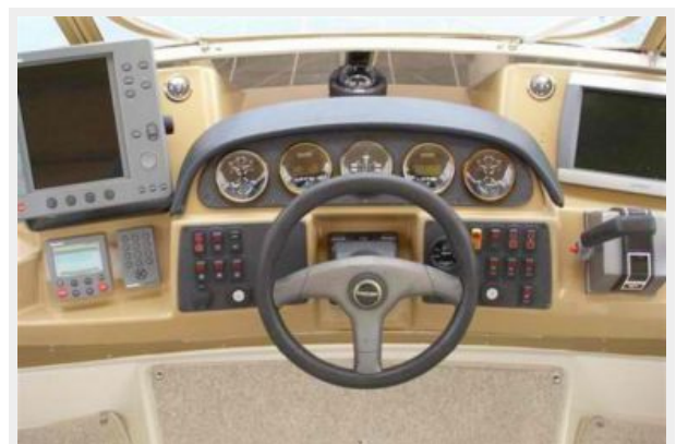
Helm with Garmin 4210 GPS and Raymarine RL80C+
