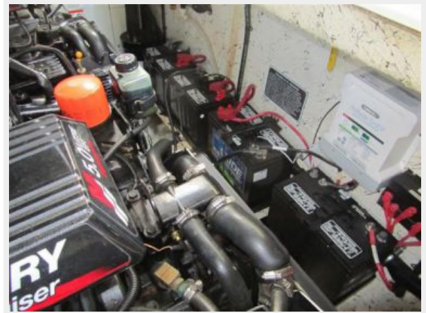
Rinker 310 Engine & house batteries
