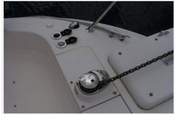
Windlass With Switches
