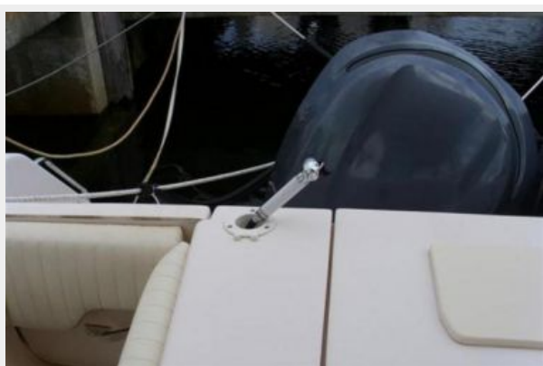
Swim Platform Fresh Water Shower
