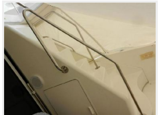
Molded Stairway to Bridge
