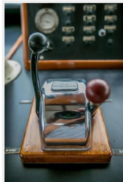
Pilot house - port throttle controls
