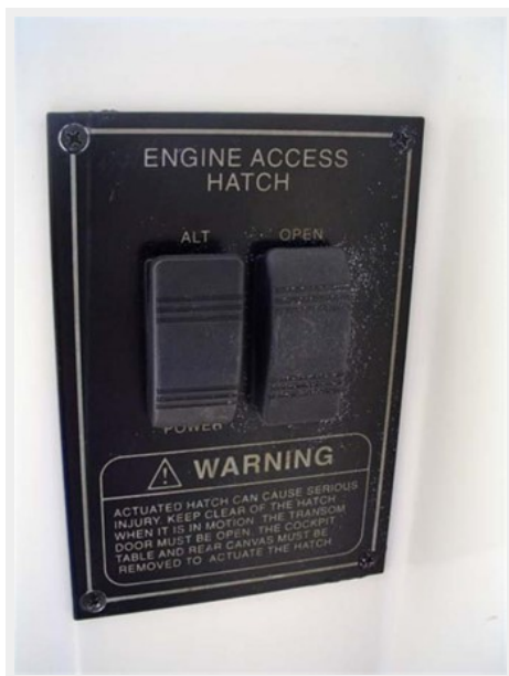
Electric Engine Hatch Rocker Switches for full access to Engine Compartment
