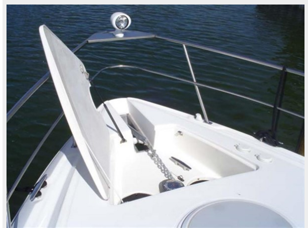
Anchor Locker with gas-assist hatch, Maxwell Windlass, Foot Pedals, with remote at helm
