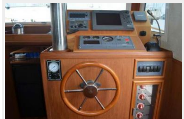
Lower helm station with Furuno chart plotter and battery switch panel made of brushed aluminum.
