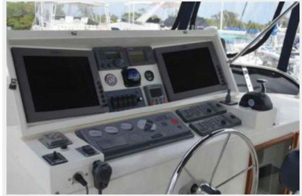
Fly bridge helm station with Furuno GPS Chartplotter, Radar, VHF, Autohelm, two (2) Flat Screen Monitors
