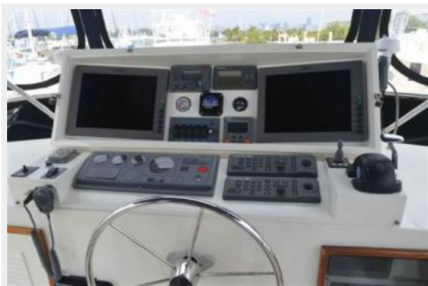
Fly bridge helm station with Furuno GPS Chartplotter, Radar, VHF, Autohelm, two (2) Flat Screen Monitors
