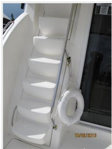
Moulded Stairs to Bridge
