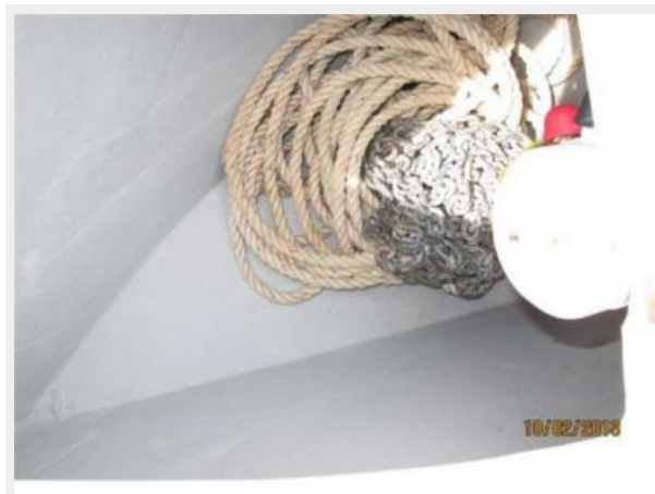
Clean Chain Locker
