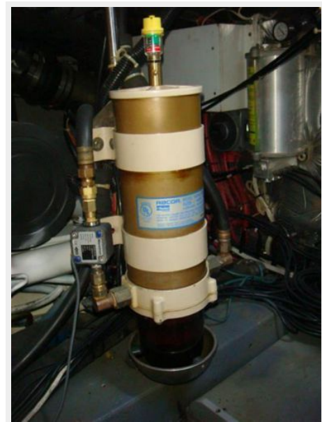
44' Carver starboard Racor fuel filter
