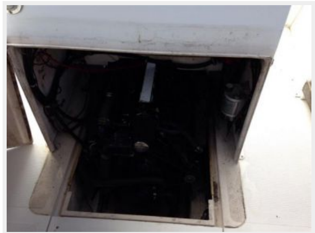
Forward console hatch removed exposing engine compartment
