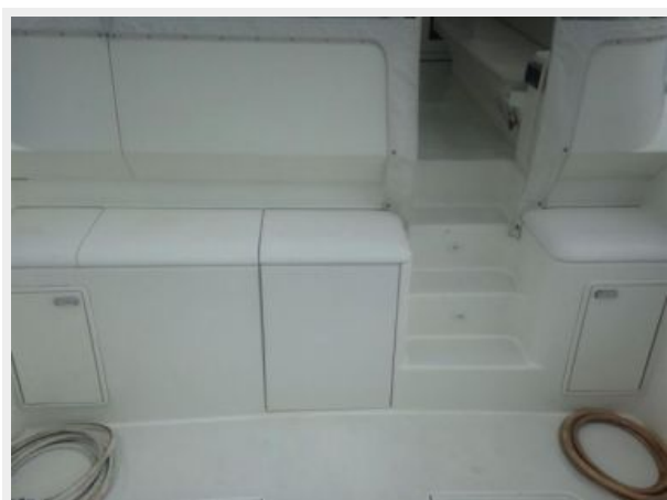
Bait prep station and engine entry door
