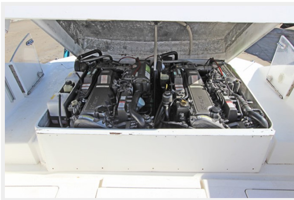
Transom Engine Compartment W/Twin 315 Yanmar Diesel Engines
