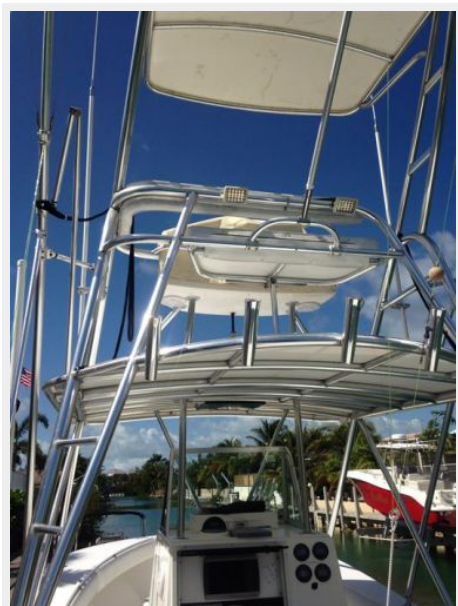
Half tower and Marlin station
