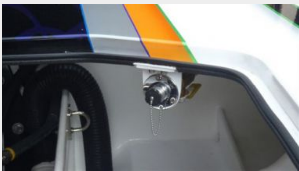
Fresh Water Flush System
