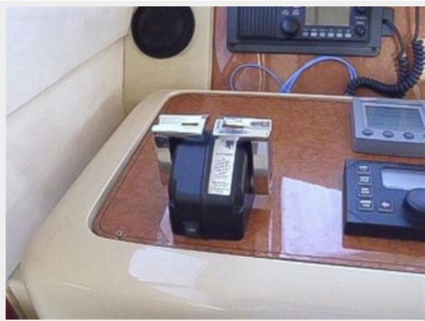
Electronic Engine Controls
