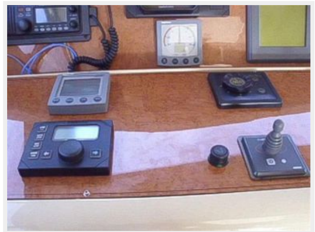
Autopilot, Combination Gauge, Remote Spotlight, Bow Thruster
