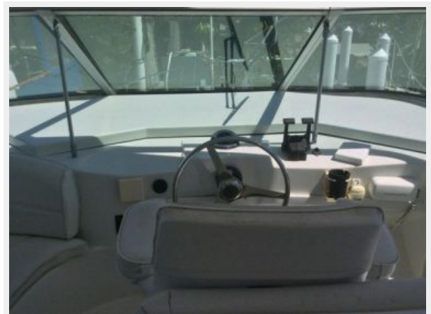
Upper Helm station with electronics lowered into console
