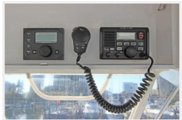
Robertson AP22 Autopilot & ICOM IC-M502 Marine VHF Radio
