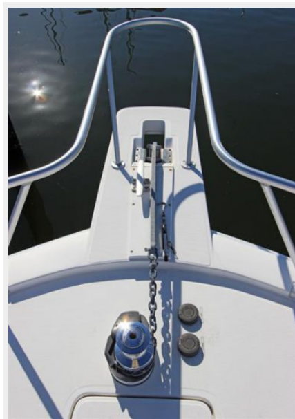
Lewmar Windlass Anchor & Bow Pulpit
