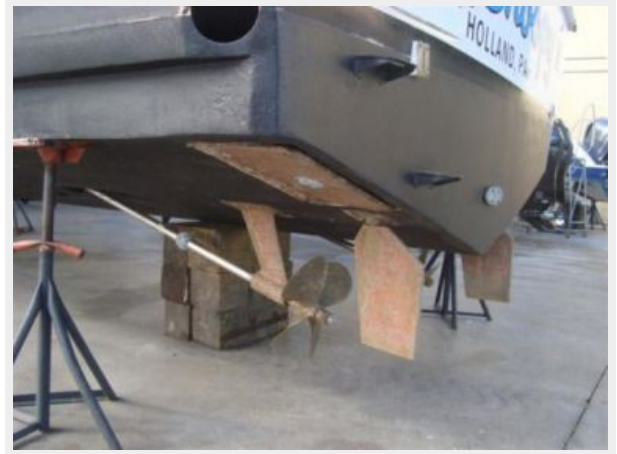
Boatyard Photo - Running Gear
