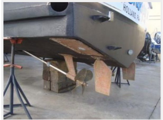
Boatyard Photo - Running Gear
