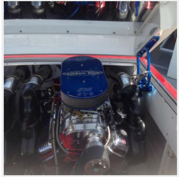
Starboard Engine w/ Blower
