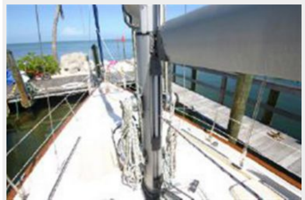
MAIN FURLER IN MAST
